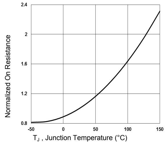
Figure 2. Normalized R<sub>DS(on)</sub> vs. T<sub>j</sub>
