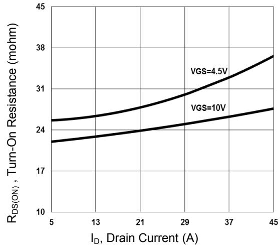
Figure 4. Turn-on Resistance vs. I<sub>D</sub>
