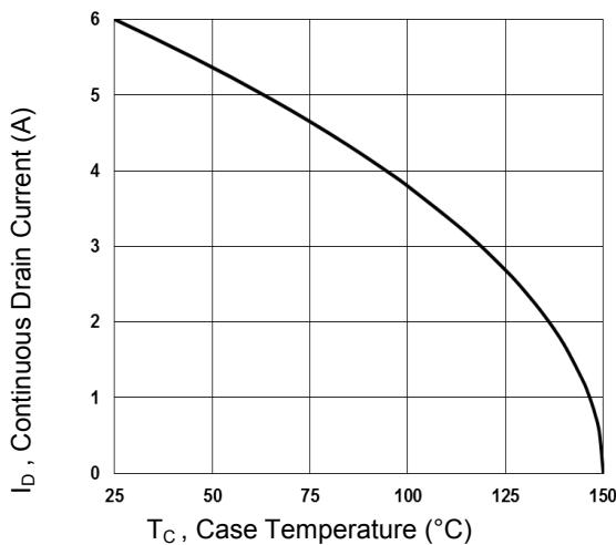
Figure 1. Continuous Drain Current vs. T<sub>c</sub>
