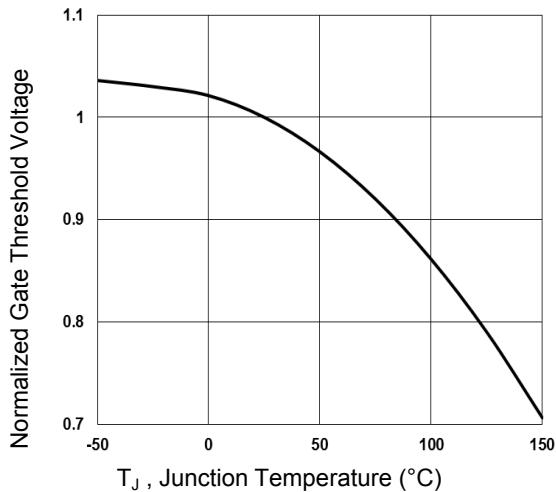
Figure 3. Normalized V<sub>th</sub> vs. T<sub>j</sub>
