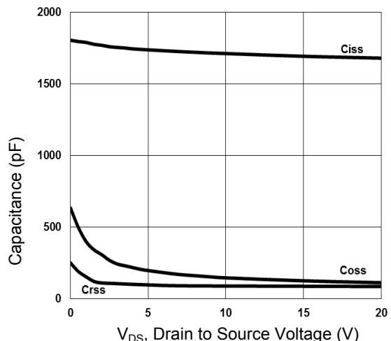
Figure \*. Capacitance Characteristics
