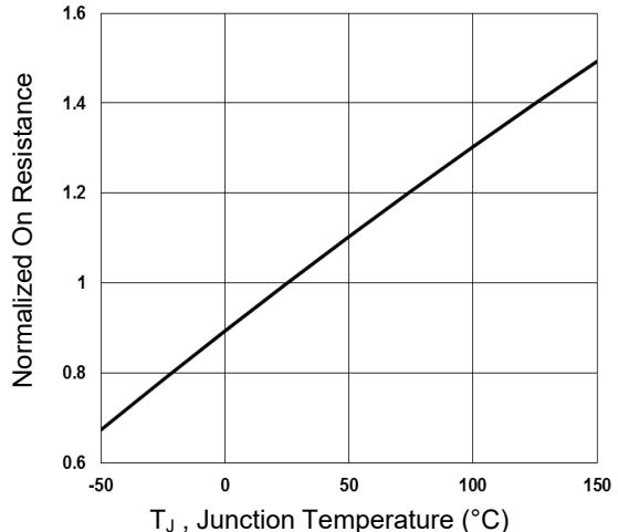
**Figure 2. Normalized R<sub>DSON</sub> vs. T<sub>j</sub>**
