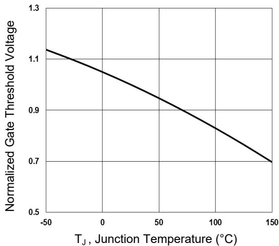
**Figure 3. Normalized V<sub>th</sub> vs. T<sub>j</sub>**
