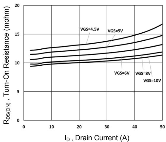
**Figure 6. Turn-On Resistance vs. I<sub>d</sub>**
