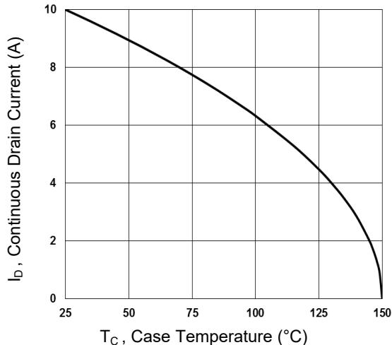
**Figure 1. Continuous Drain Current vs. T<sub>c</sub>**
