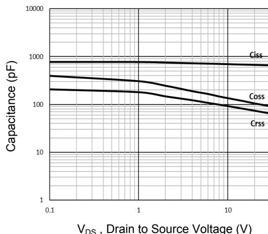
Figure 7. Capacitance Characteristics
