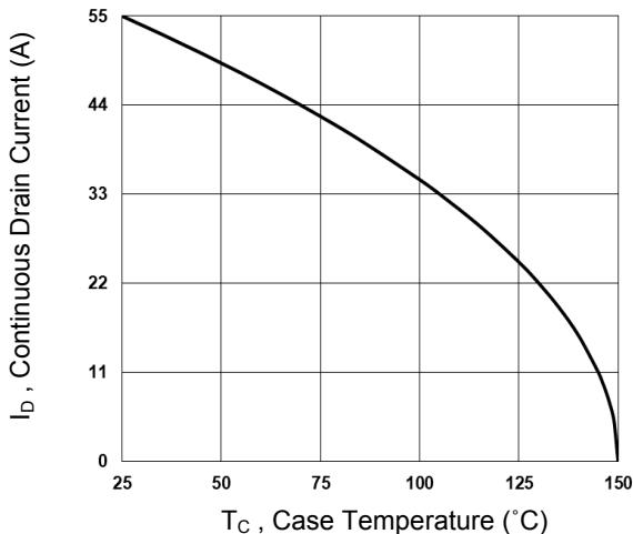
Figure 1. Continuous Drain Current vs. T<sub>c</sub>
