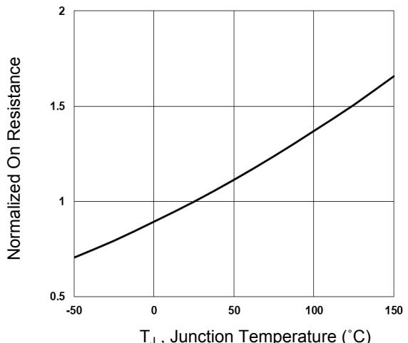
Figure 2. Normalized R<sub>DS(ON)</sub> vs. T<sub>j</sub>
