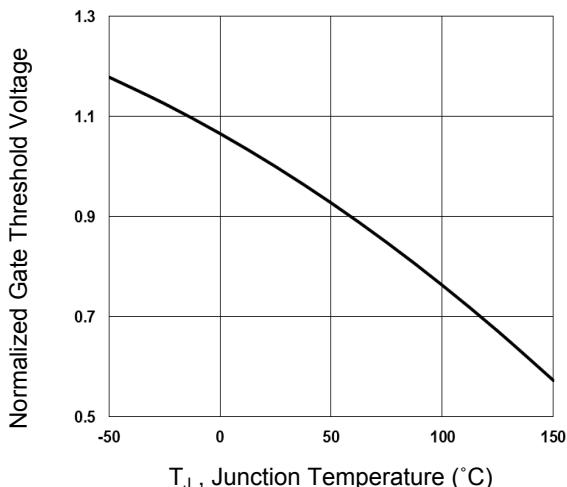
Figure 3. Normalized V<sub>th</sub> vs. T<sub>j</sub>
