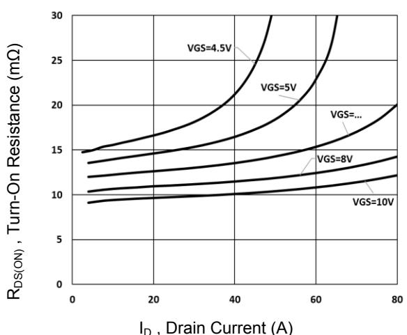
Figure 6. Turn-On Resistance vs. I<sub>D</sub>
