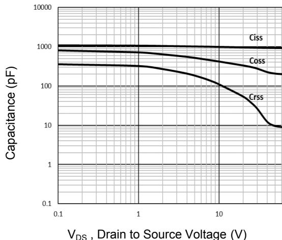
Figure 7. Capacitance Characteristics
