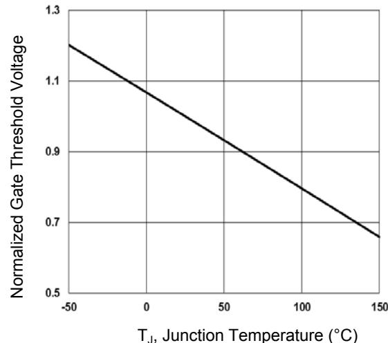
Figure 3. Normalized V<sub>th</sub> vs. T<sub>j</sub>
