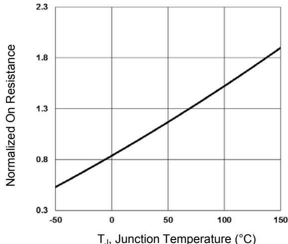
Figure 2. Normalized R<sub>DS(ON)</sub> vs. T<sub>j</sub>
