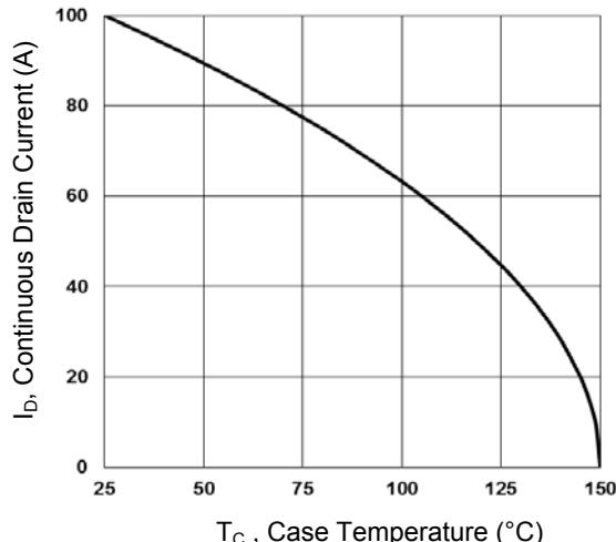
Figure 1. Continuous Drain Current vs. T<sub>c</sub>
