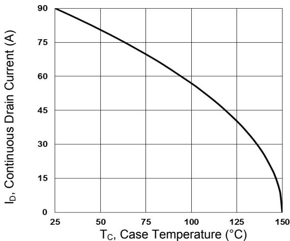
Figure 1. Continuous Drain Current vs. T<sub>c</sub>
