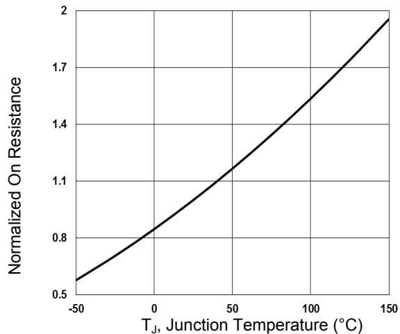
Figure 2. Normalized R<sub>DS(ON)</sub> vs. T<sub>j</sub>
