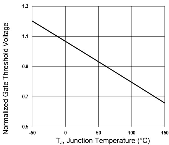
Figure 3. Normalized V<sub>th</sub> vs. T<sub>j</sub>
