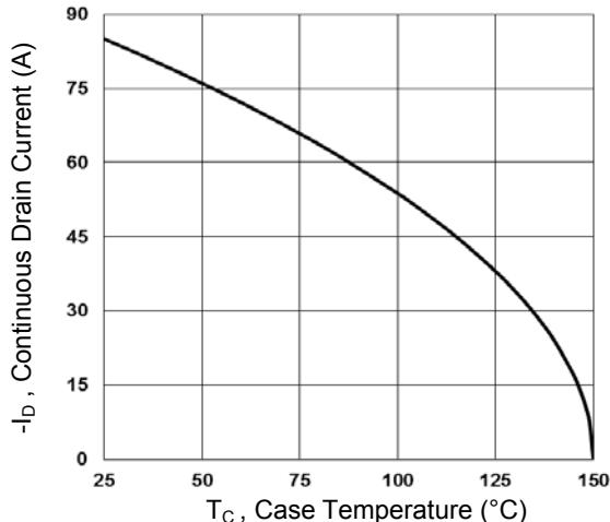
Figure 1. Continuous Drain Current vs. T<sub>c</sub>
