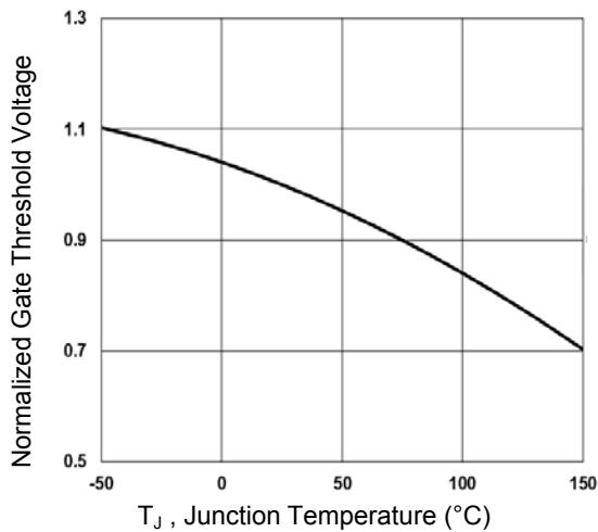
Figure 3. Normalized V<sub>th</sub> vs. T<sub>j</sub>
