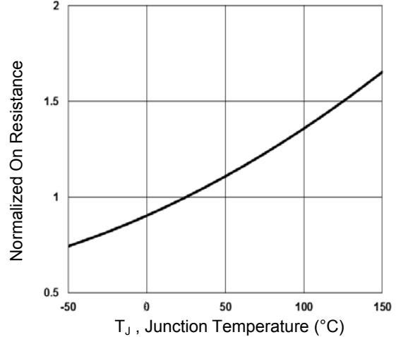
Figure 2. Normalized R<sub>DS(ON)</sub> vs. T<sub>j</sub>
