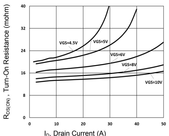
Figure 6. Turn-on Resistance vs. I<sub>D</sub>
