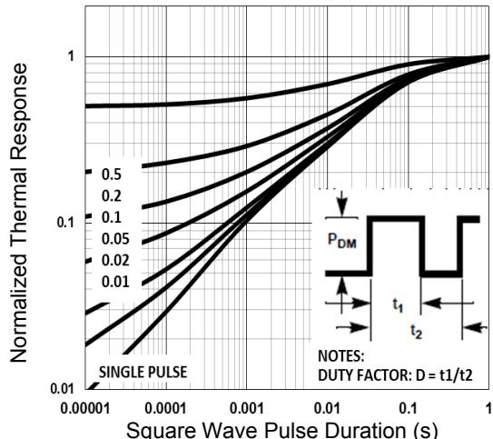
Figure 8. Normalized Transient Response
