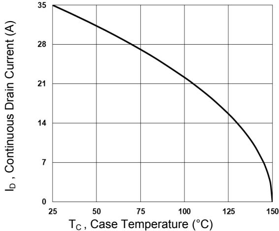
Figure 1. Continuous Drain Current vs. T<sub>C</sub>
