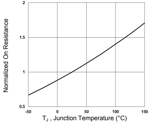
Figure 2. Normalized R<sub>DS(on)</sub> vs. T<sub>J</sub>
