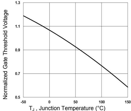
Figure 3. Normalized V<sub>th</sub> vs. T<sub>J</sub>
