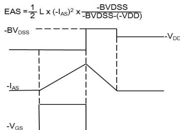
**Fig.8**  $E_{AS}$  Waveform
