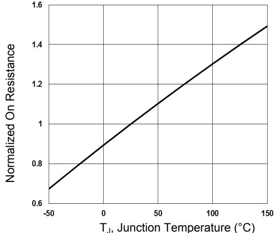
Figure 2. Normalized R<sub>DS(ON)</sub> vs. T<sub>J</sub>
