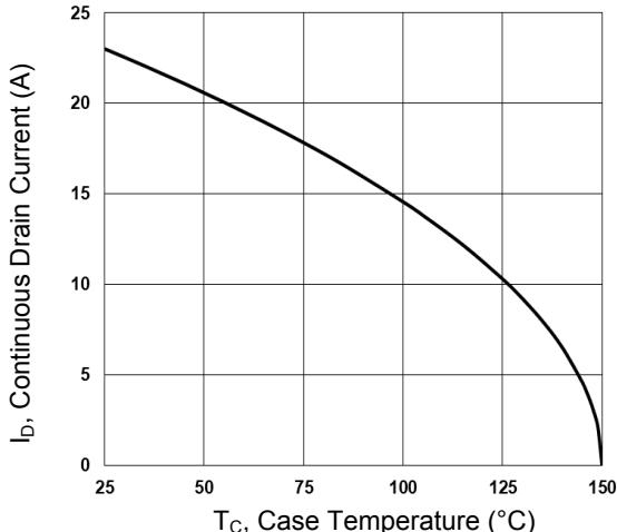
Figure 1. Continuous Drain Current vs. T<sub>C</sub>
