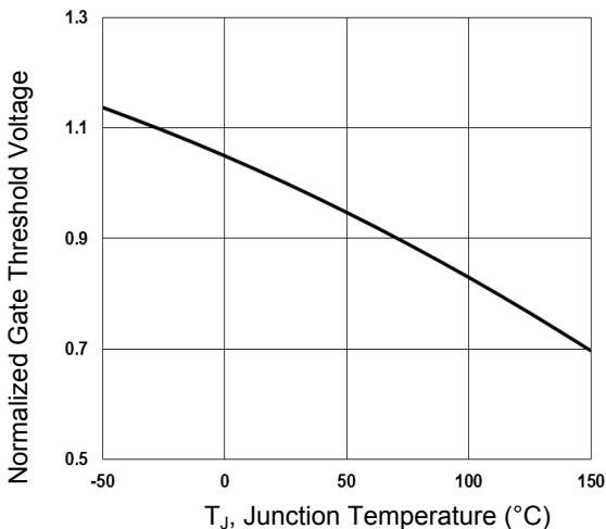
Figure 3. Normalized V<sub>th</sub> vs. T<sub>J</sub>
