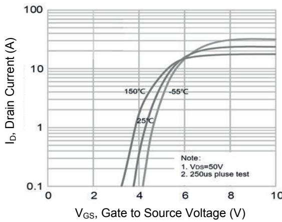
Figure 2. Transfer Characteristics
