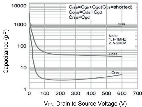
**Figure 7. Capacitance Characteristics**
