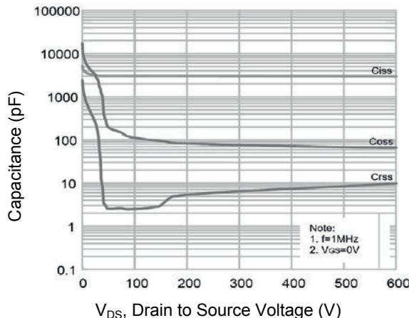
**Figure 7. Capacitance Characteristics**
