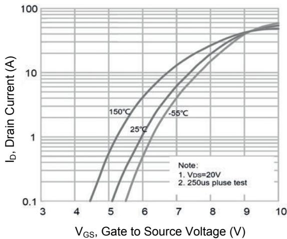
Figure 2. Transfer Characteristics
