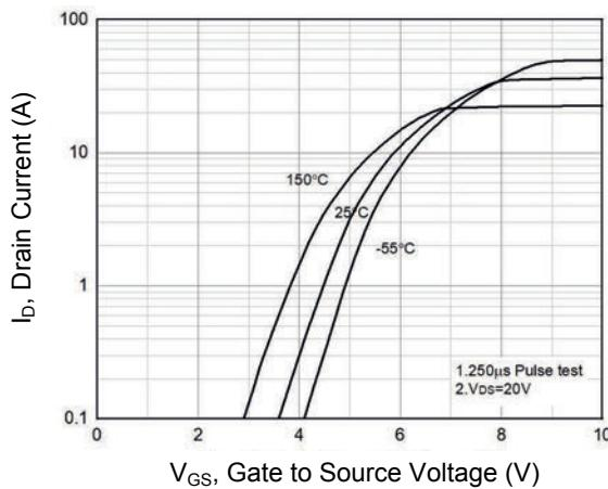
**Figure 3. Transfer Characteristics**
