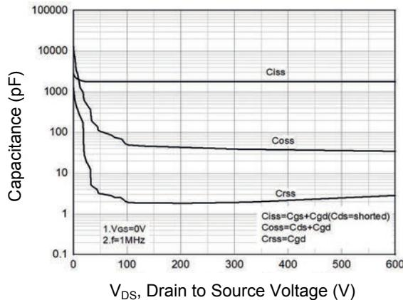
**Figure 7. Capacitance Characteristics**
