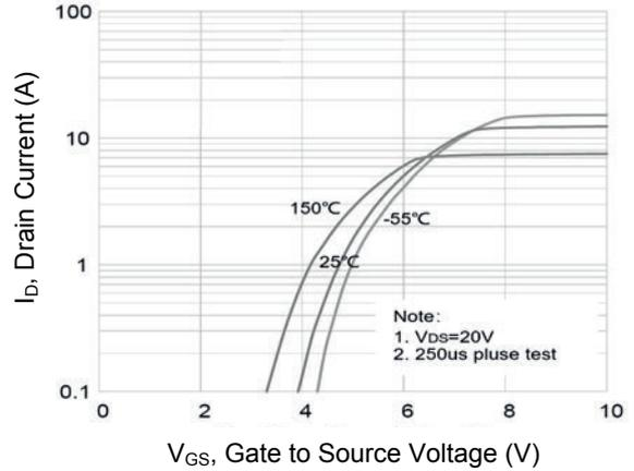
Figure 2. Transfer Characteristics
