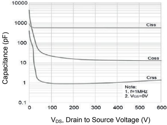
**Figure 7. Capacitance Characteristics**
