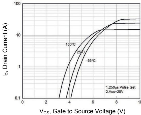
**Figure 3. Transfer Characteristics**
