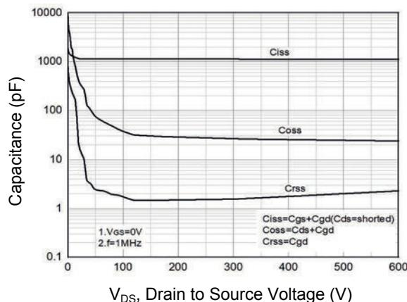
Figure 7. Capacitance Characteristics
