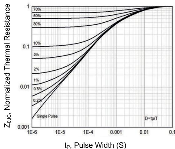
Figure 15. Transient Thermal Impedance Vs. t<sub>P</sub>
