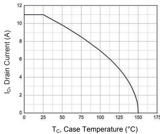
Figure 14. Drain Current Vs. T<sub>c</sub>
