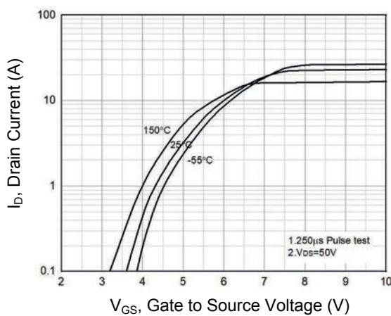
**Figure 3. Transfer Characteristics**
