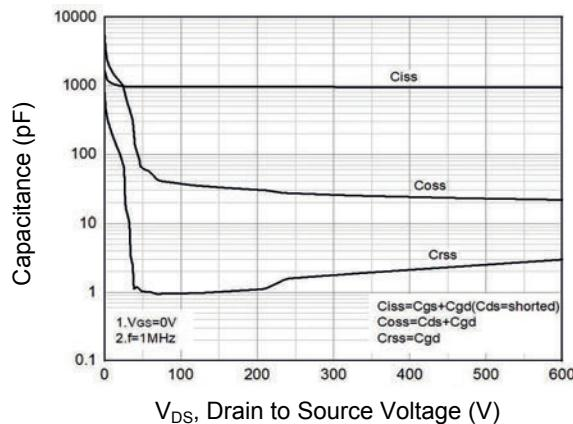
**Figure 7. Capacitance Characteristics**
