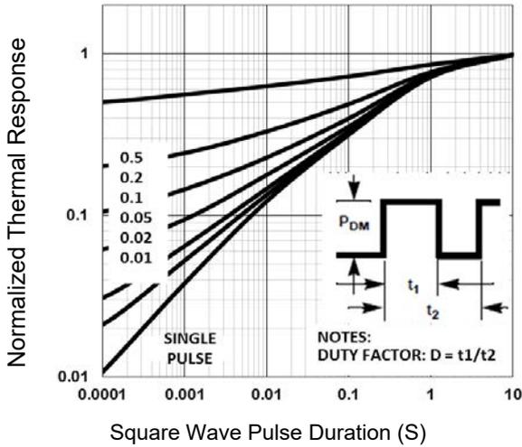
**Figure 9. Normalized Trtransient Impedance**
