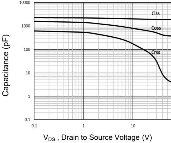
**Figure 7. Capacitance Characteristics**
