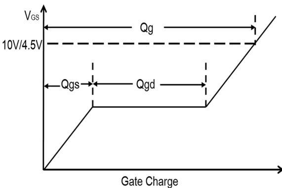
**Figure 11. Gate Charge Waveforms**
