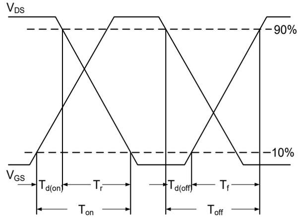
**Figure 12. Switch Time Waveforms**
