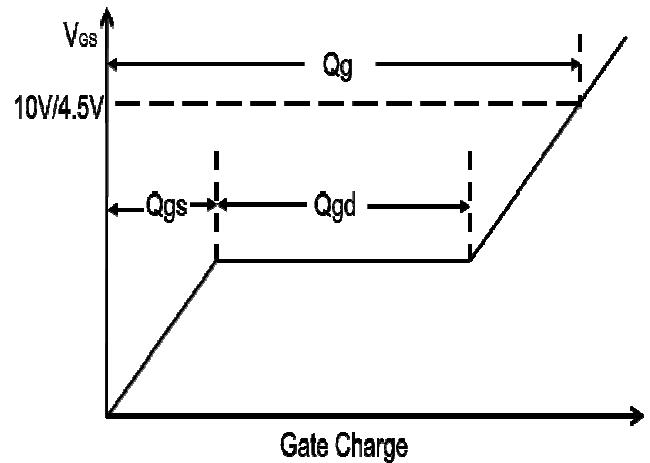
Figure 8. Gate Charge Waveform
