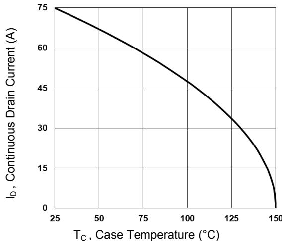
Figure 1. Continuous Drain Current vs. T<sub>c</sub>
