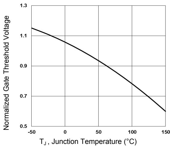
Figure 3. Normalized V<sub>th</sub> vs. T<sub>j</sub>
