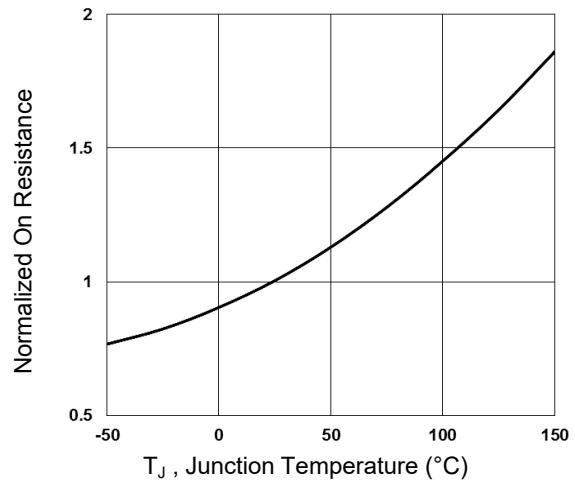
Figure 2. Normalized R<sub>DSON</sub> vs. T<sub>j</sub>
