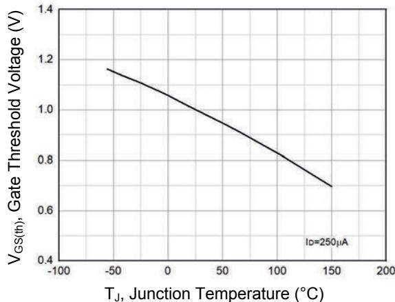
Figure 11. Gate Threshold Voltage Vs.  $T_J$
