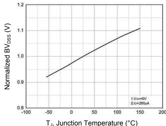
Figure 12. Normalized  $BV_{DSS}$  Vs.  $T_J$
