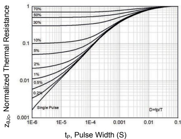
Figure 15. Transient Thermal Impedance Vs. t<sub>p</sub>
