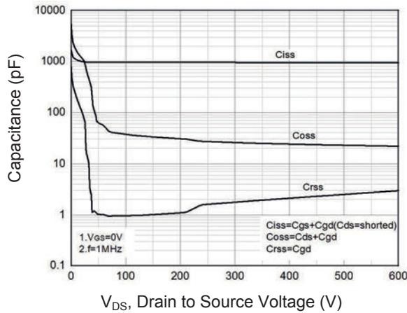
Figure 7. Capacitance Characteristics
