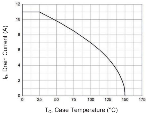
Figure 14. Drain Current Vs. T<sub>c</sub>
