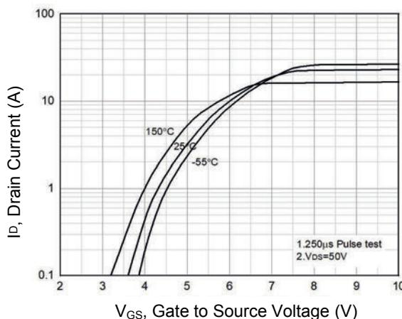
Figure 3. Transfer Characteristics
