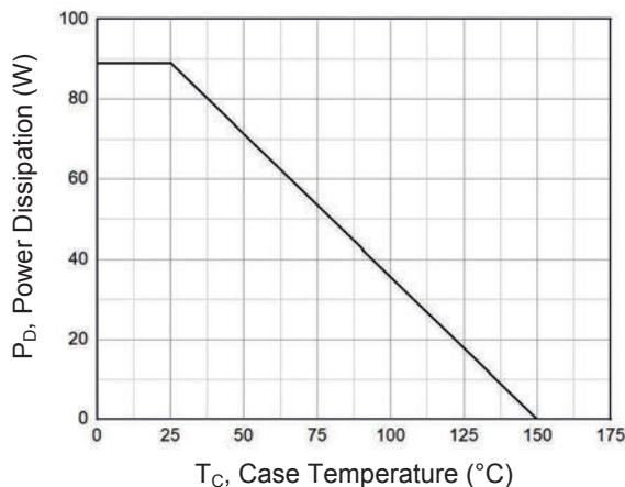
Figure 13. Power Dissipation Vs. T<sub>c</sub>
