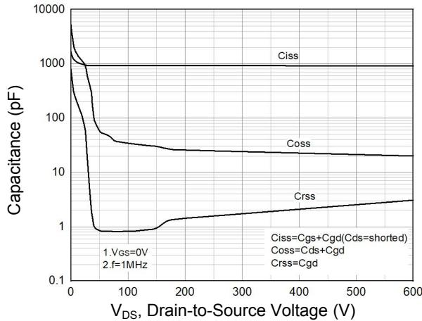
Figure 7. Capacitance Characteristics
