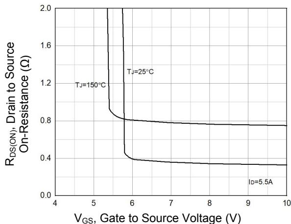
Figure 9. On Resistance vs.  $V_{GS}$
