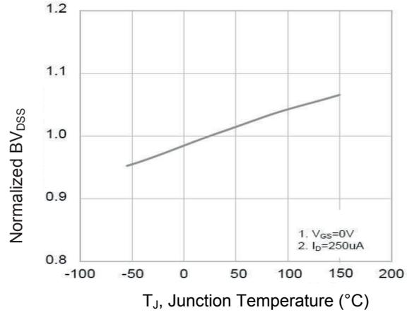
**Figure 8. Normalized  $BV_{DS}$  Vs.  $T_J$**
