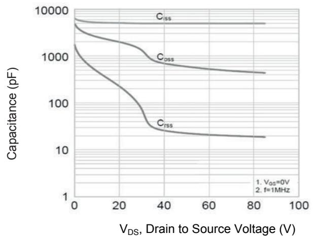
**Figure 6. Typical Capacitance Vs. Drain to Source Voltage**
