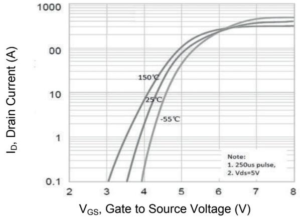
**Figure 2. Transfer Characteristics**
