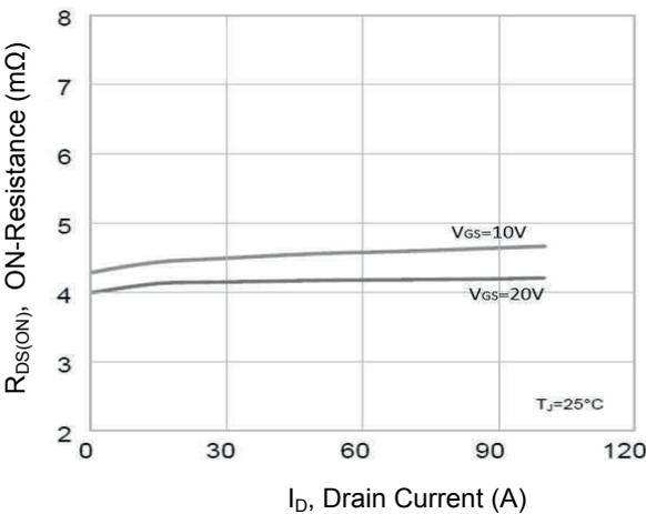
**Figure 5. On-Resistance vs. Drain Source**
