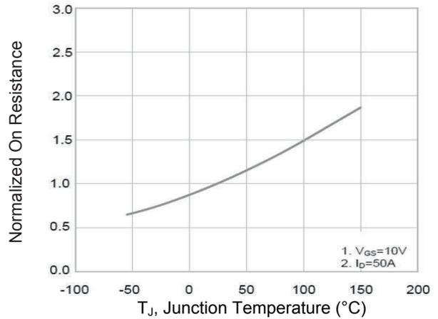
**Figure 4. Normalized On-Resistance Vs.  $T_J$**
