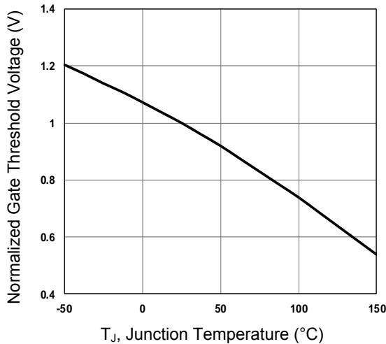
**Figure 3. Normalized V<sub>th</sub> vs. T<sub>j</sub>**
