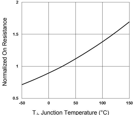
**Figure 2. Normalized R<sub>DSON</sub> vs. T<sub>j</sub>**
