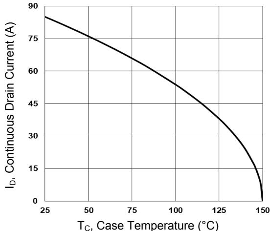
**Figure 1. Continuous Drain Current vs. T<sub>c</sub>**
