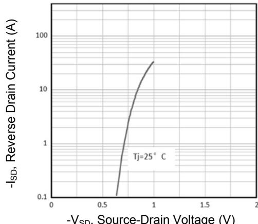
Figure 5. Typical Source-Drain Diode Forward Voltage
