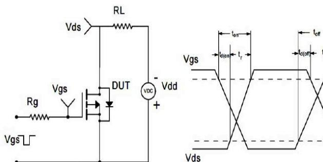
Figure 10. Switching Time Test Circuit and Waveforms
