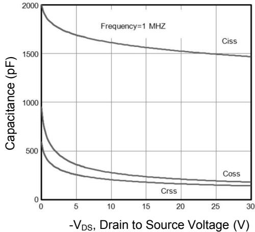
Figure 7. Capacitance Characteristics
