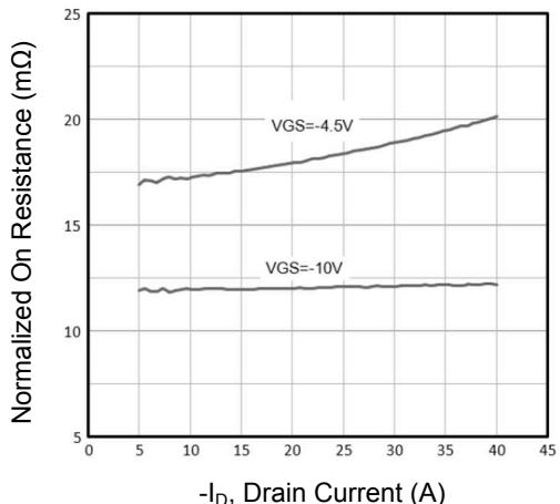
Figure 4. Normalized  $R_{DS(ON)}$  vs.  $I_D$
