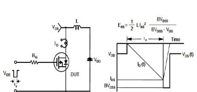
Figure 11. Unclamped Inductive Test Circuit and Waveforms
