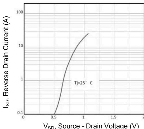
Figure 5. Typical Source - Drain Diode Forward Voltage
