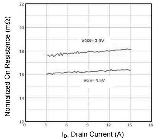
Figure 4. Normalized  $R_{DS(\text{ON})}$  vs.  $I_D$
