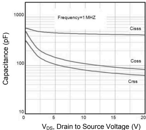
Figure 7. Capacitance Characteristics
