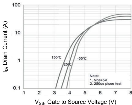
Figure 2. Transfer Characteristics
