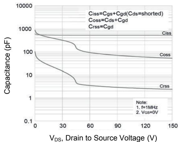
Figure 7. Capacitance Characteristics
