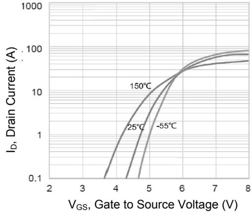
**Figure 2. Transfer Characteristics**
