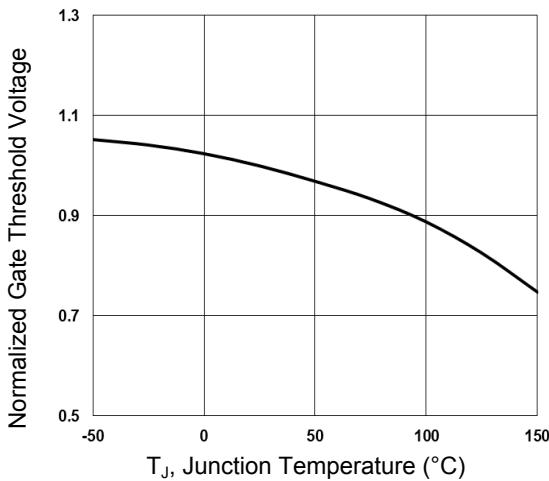
Figure 3. Normalized V<sub>th</sub> vs. T<sub>J</sub>
