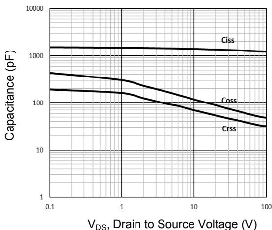
Figure 7. Capacitance Characteristics
