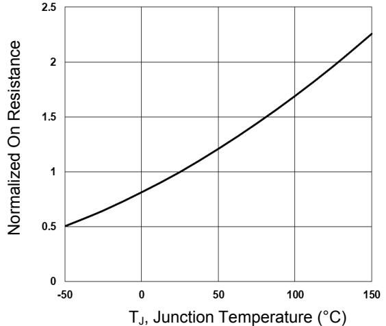
Figure 2. Normalized R<sub>DS(on)</sub> vs. T<sub>J</sub>
