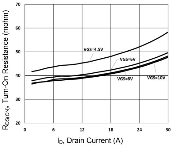
Figure 6. Turn-On Resistance vs. I<sub>D</sub>
