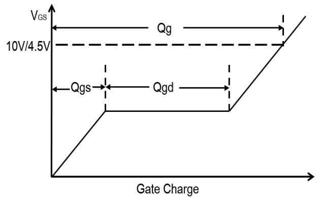
Figure 11. Gate Charge Waveform
