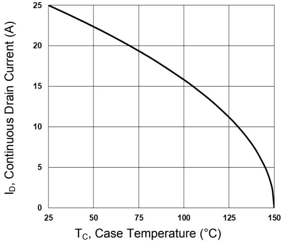
Figure 1. Continuous Drain Current vs. T<sub>C</sub>
