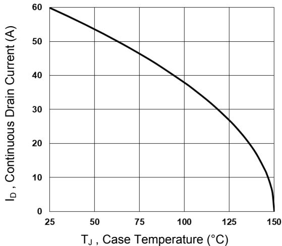
Fig.1 Continuous Drain Current vs. T<sub>c</sub>
