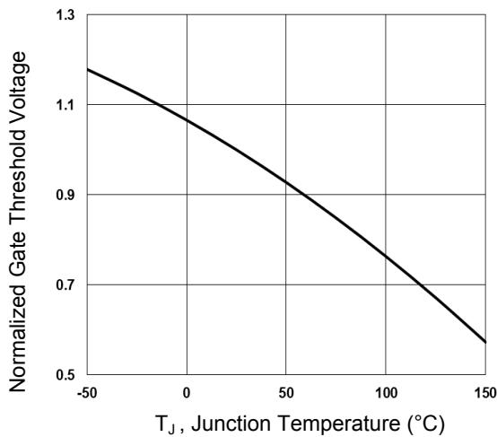
Fig.3 Normalized V<sub>th</sub> vs. T<sub>J</sub>
