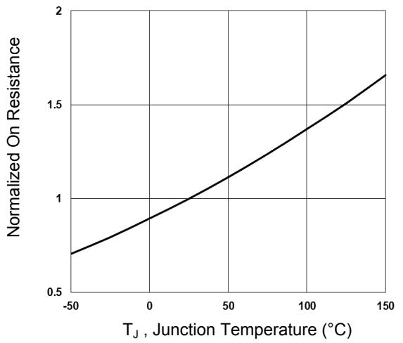
Fig.2 Normalized R<sub>DS(ON)</sub> vs. T<sub>J</sub>
