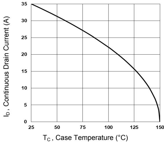
Figure 1. Continuous Drain Current vs. T<sub>c</sub>
