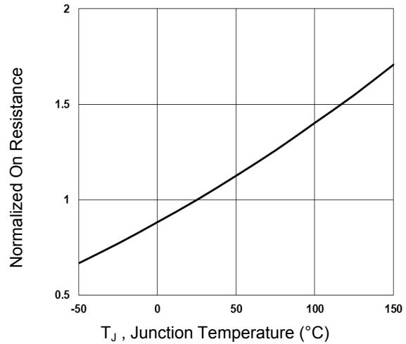
Figure 2. Normalized R<sub>DSON</sub> vs. T<sub>j</sub>
