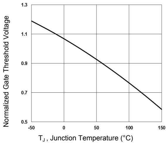
Figure 3. Normalized V<sub>th</sub> vs. T<sub>j</sub>
