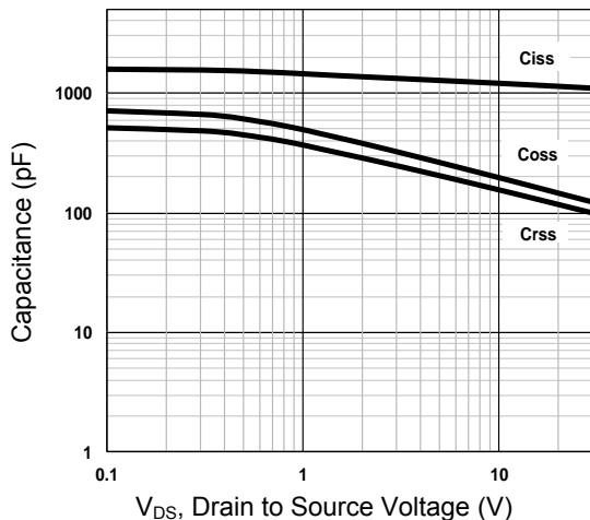
Figure 7. Capacitance Characteristics
