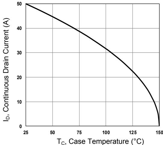
Figure 1. Continuous Drain Current vs. T<sub>c</sub>
