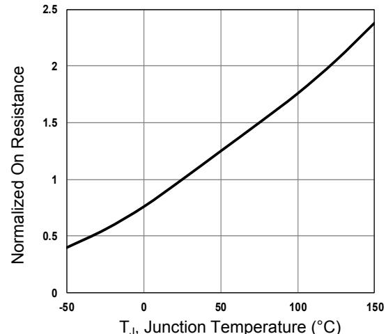
Figure 2. Normalized R<sub>DSON</sub> vs. T<sub>j</sub>
