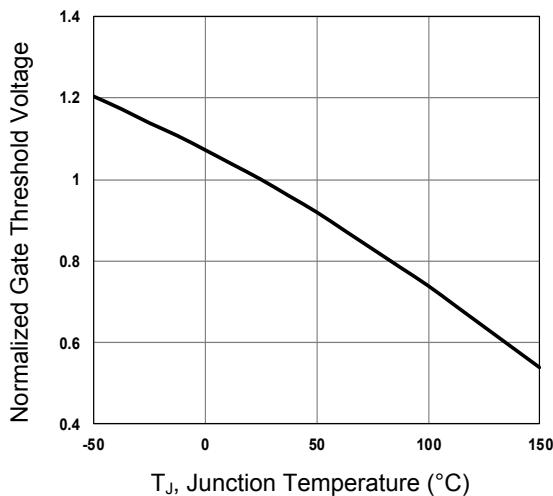
Figure 3. Normalized V<sub>th</sub> vs. T<sub>j</sub>
