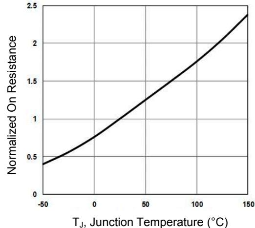
Figure 2. Normalized R<sub>DSON</sub> vs. T<sub>J</sub>
