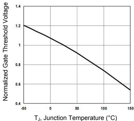
Figure 3. Normalized V<sub>th</sub> vs. T<sub>J</sub>
