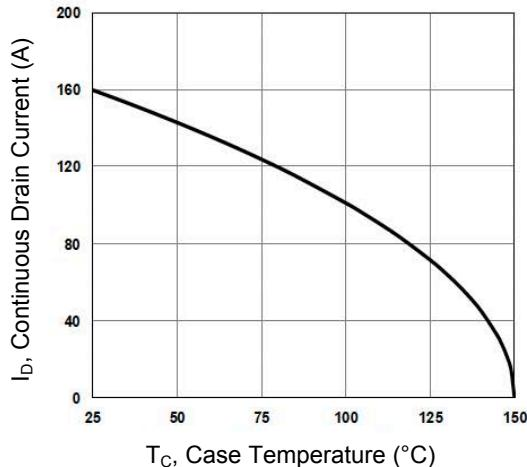
Figure 1. Continuous Drain Current vs. T<sub>C</sub>
