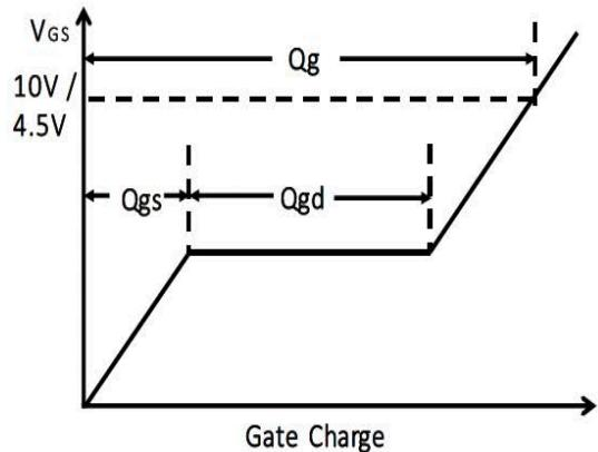
Figure 8. Gate Charge Waveform
