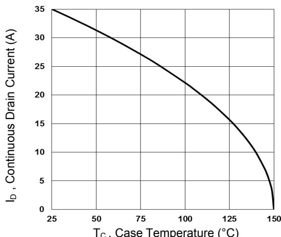
Figure 1. Continuous Drain Current vs. T<sub>c</sub>
