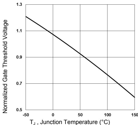
Figure 3. Normalized V<sub>th</sub> vs. T<sub>j</sub>
