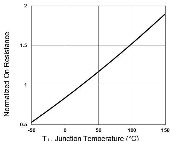
Figure 2. Normalized R<sub>DS(ON)</sub> vs. T<sub>j</sub>
