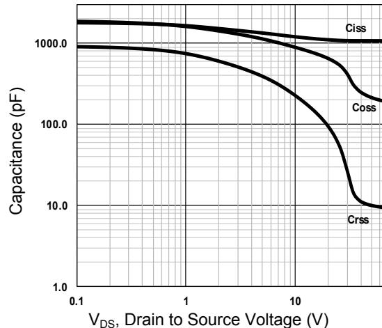
Figure 7. Capacitance Characteristics
