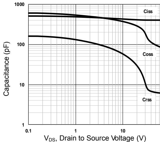
Figure 7. Capacitance Characteristics
