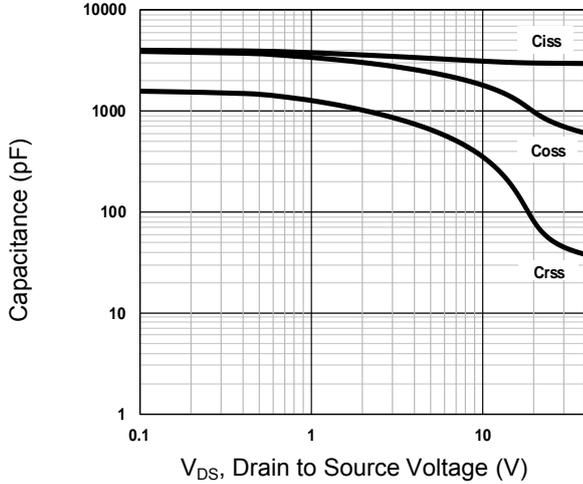
**Figure 7. Capacitance Characteristics**
