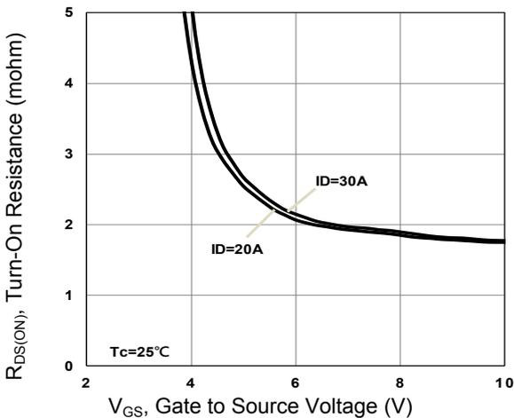
**Figure 5. Turn-On Resistance vs.  $V_{GS}$**
