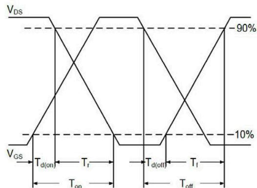
Figure 11. Switching Time Waveform
