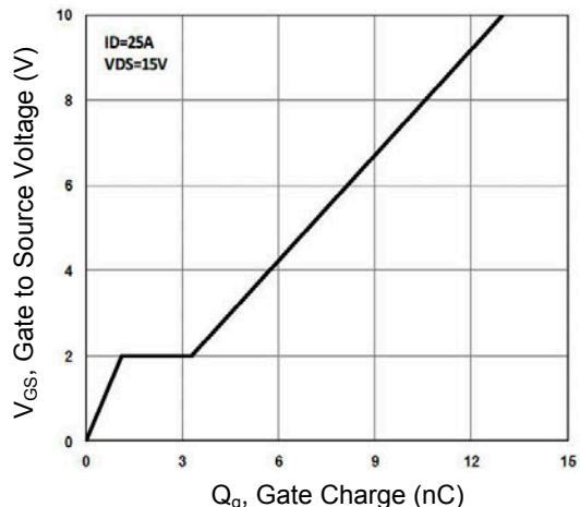
Figure 8. Gate Charge Waveform
