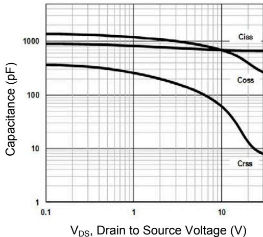
Figure 7. Capacitance Characteristics
