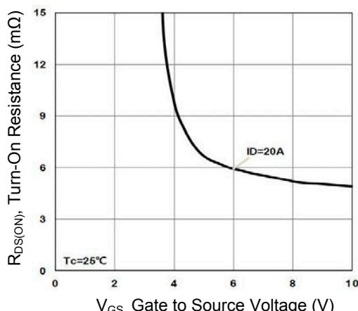
Figure 5. Turn-On Resistance vs.  $V_{GS}$
