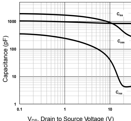
Figure 7. Capacitance Characteristics
