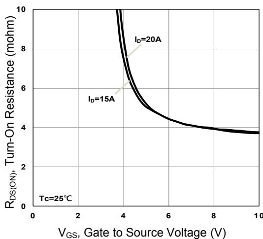
Figure 5. Turn-On Resistance vs.  $V_{GS}$
