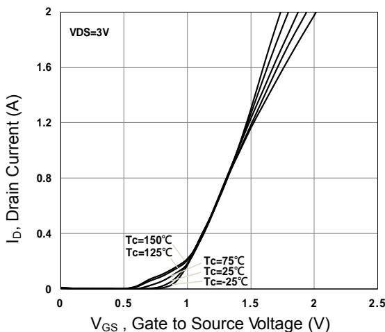
Figure 9. Transfer Characteristics
