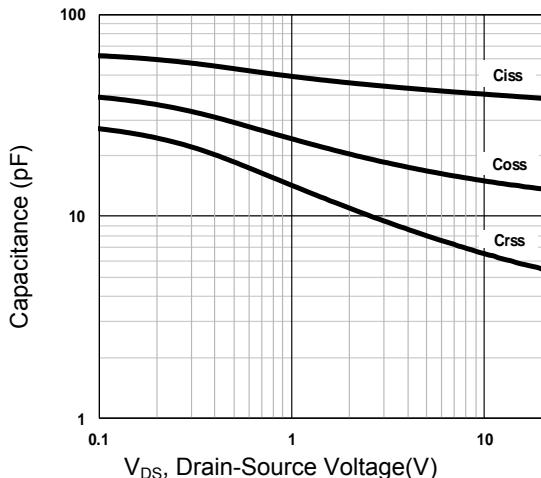
Figure 7. Capacitance Characteristics
