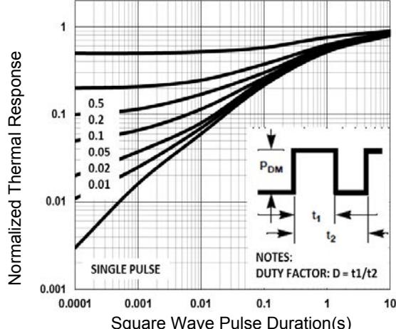
Figure 11. Normalized Transient Impedance
