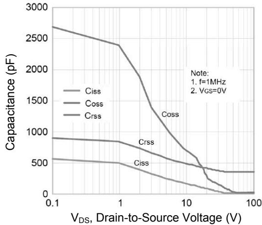
Figure 7. Capacitance Characteristics
