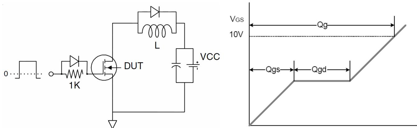
Figure 13. Gate Charge Test Circuit and waveforms
