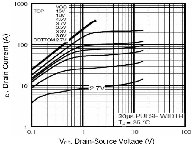
**Figure 1. Output Characteristics**
