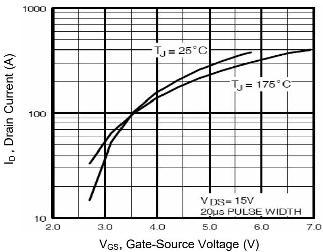
**Figure 3. Transfer Characteristics**
