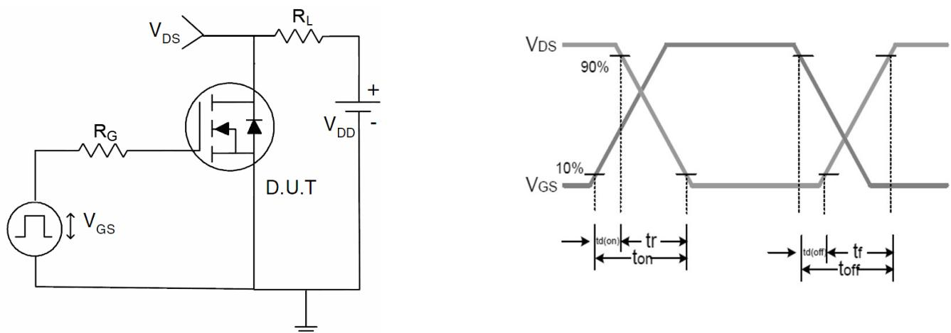
Figure 14. Switch Time Test Circuit and waveforms
