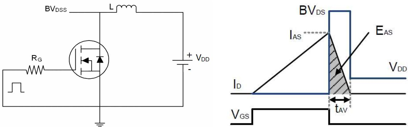
Figure 12. E<sub>AS</sub> Test Circuit and waveforms
