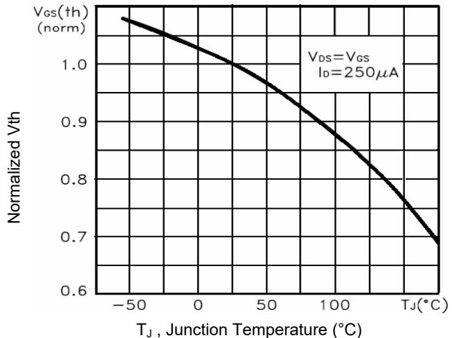
Figure 10.  $V_{th}$  Vs. Junction Temperature
