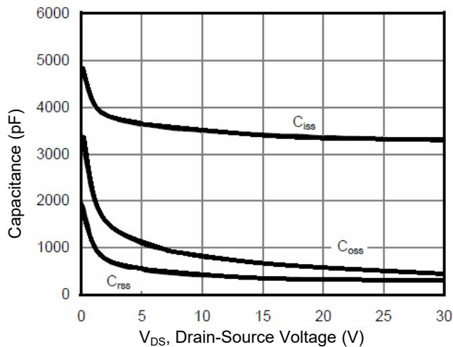
Figure 7. Capacitance Characteristics
