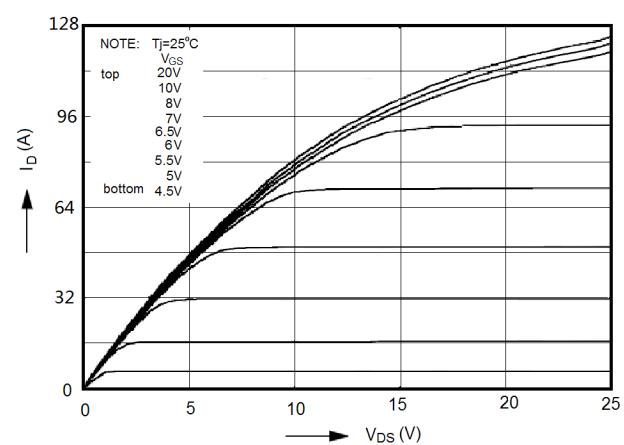
Figure 4. Output Characteristics
