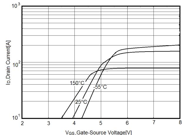
Figure 5. Transfer Characteristics
